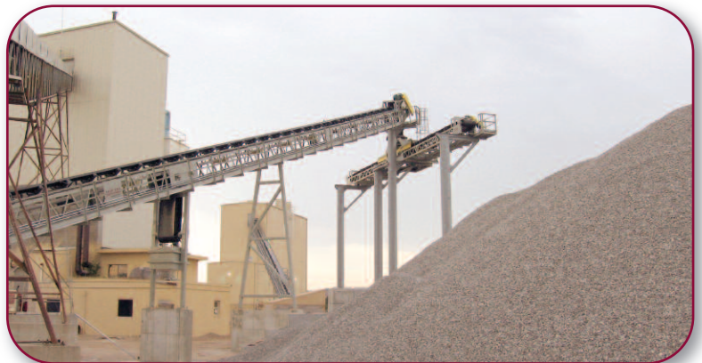
30" x 200' Stationary Truck Unloading Conveyor feeding (2) 30" x 31' Stationary Conveyors
