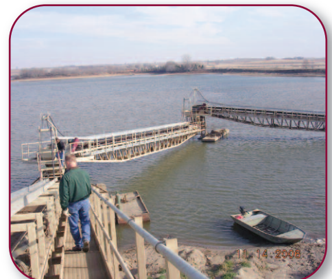
Multiple 42" x 100' Floating Conveyor sections with full length catwalk and rotating transition points
