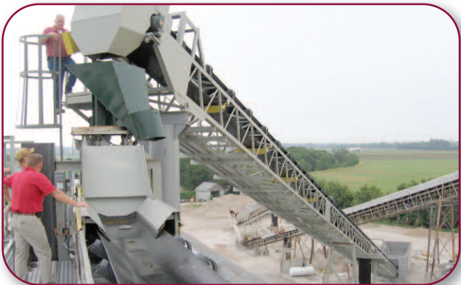
30" x 200' Stationary Truck Unloading Conveyor feeding (2) 30" x 31' Stationary Conveyors
