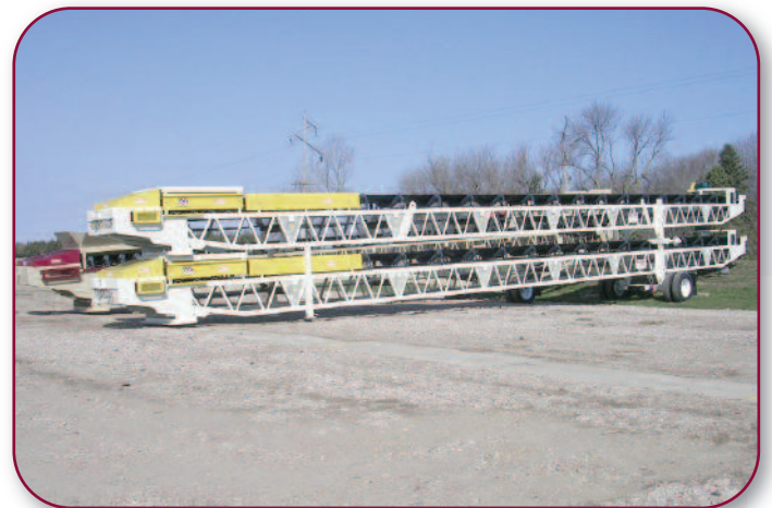
36" X 80' (2) Stack-up Transfer Conveyors
