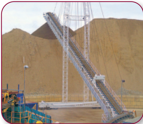
48" x 220' Radial Mast Stacking Conveyor
