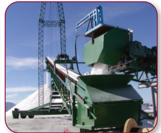
42" x 230' Radial Mast Stacking Conveyor
