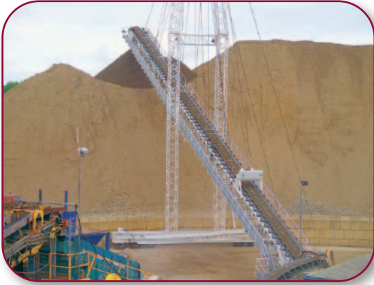
42" x 220' Mast-Type Radial Stacker System with full length catwalk
