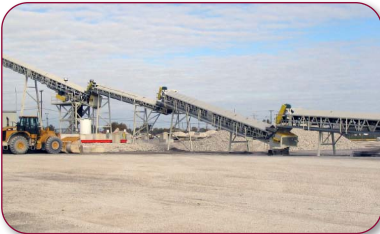
42" x 96' (3) Stationary Transfer Conveyors
