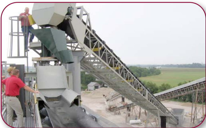
30" x 200' Stationary Truck Unloading Conveyor feeding two 30" x 31' Stationary Conveyors
